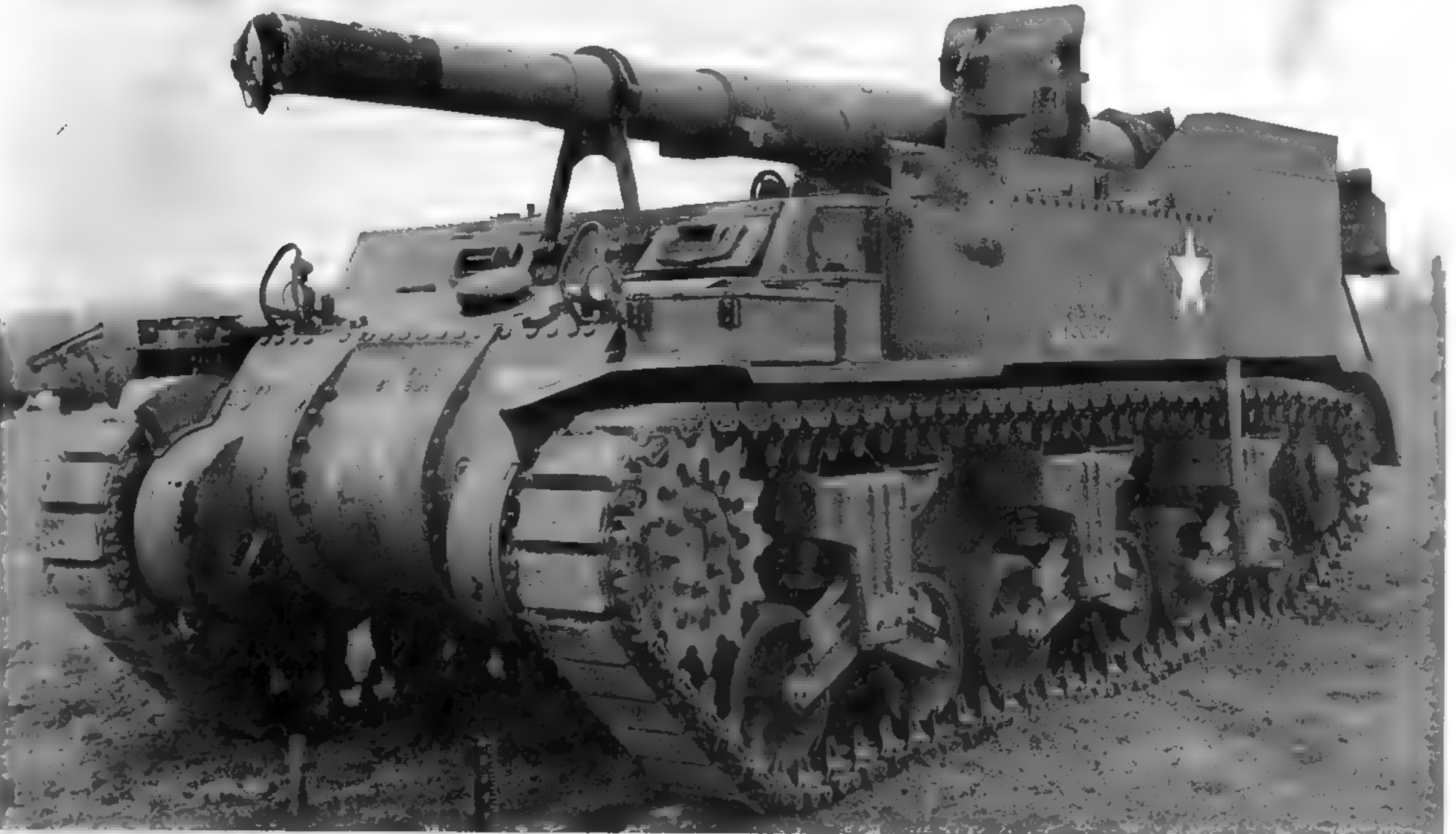
The M12 was the Army's first successful attempt at a 155mm self-propelled gun. The chassis was based on that of the M3 medium tank, with some modifications. (Photo courtesy of the Patton Museum)
